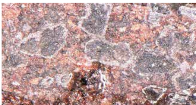
Grinding wheel surface before erosive processing
